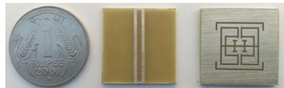
Fig.7 Fabricated CSRR loaded transmission line (a)Top view (microstrip line) (b) Bottom view (CSRR)
